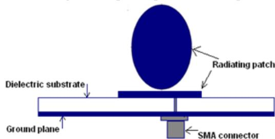
Figure 1 Side and top view with feed arrangement of designed elliptical patch antenna
