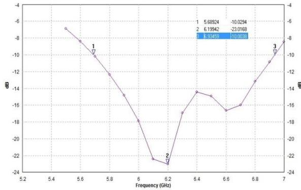
Figure 4 Simulated reflection coefficient of modified assembly of patches
