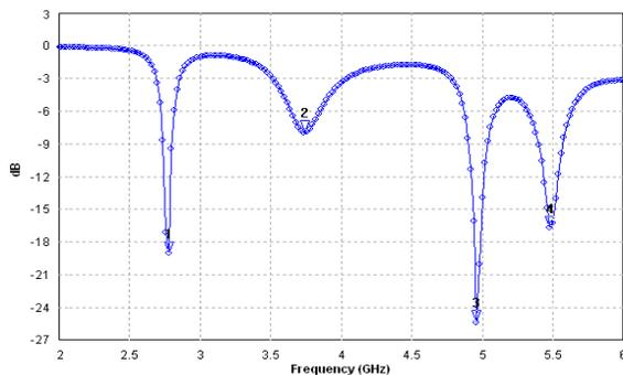
Figure 2 Simulated reflection coefficient of EPMA
