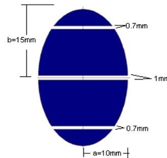
Figure 3 Designed Gap-Coupled Assembly of Patches forming Elliptical Microstrip Patch Antenna
