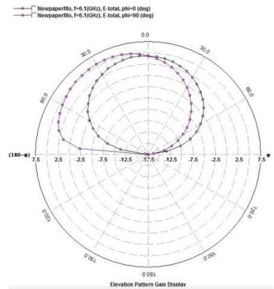
Figure 8 Simulated elevation patterns at the frequency 6.2 GHz.
