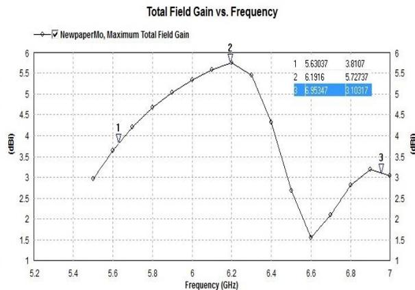
Figure 5 Simulated result of total Field Gain V/s Frequency
