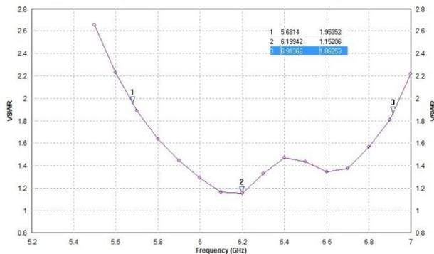
Figure 6 Simulated VSWR for modified assembly of patches with frequency
